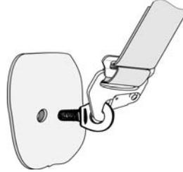
The eye bolt must be positioned so the snap-on bracket can hook into the eye with enough freedom for the bracket to move into the direction of pull. The snap-on bracket must be allowed to fully align with the webbing routing when loaded.
