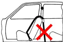
Never install shoulder belts directly to the floor behind the seat!
